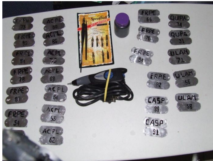
Fig. 4 — Engraved aluminum tags, Dremel engraver, and calligraphy pen used for permanent tag fabrication.
